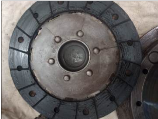
Plenty left on the clutch plate but clearly there is oil coming from somewhere.
