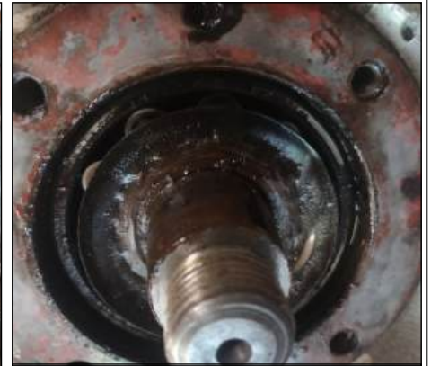
Cover plate off and the oil thrower is clearly not doing its job.
