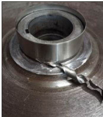
The lower rim now needed to be removed. A slot had been machined around the sleeve but removal was still much more difficult than I thought it would be.
