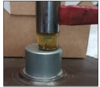
A cap to fit the sleeve is supplied and it was an excellent fit on the Flywheel Boss. Sigh of relief!!!
