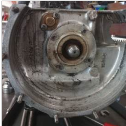
Flywheel off and it looks like the oil is coming from the main bearing area.
