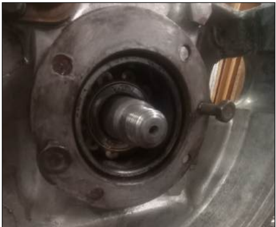
The outer race was withdrawn, luckily the threads in the retaining plate were OK.
