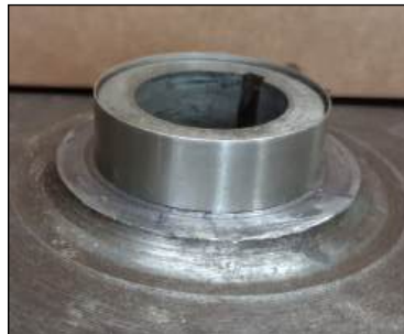
I used a piece of hardwood and hammer to fully drive the sleeve down once the lip was fully removed. But it still stood proud of the boss.
