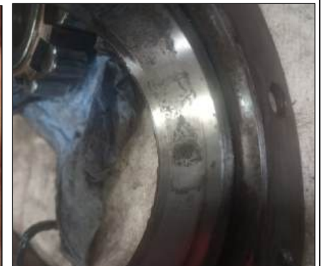
The rollers and outer race were found to be very badly worn and unusable.
