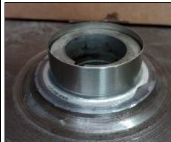
The lower rim now needed to be removed. A slot had been machined around the sleeve but removal was still much more difficult than I thought it would be.
