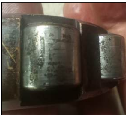
The rollers and outer race were found to be very badly worn and unusable.
