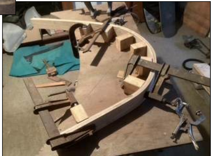
Laminating wheel arches.
