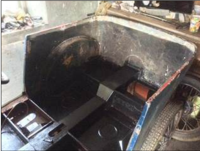
Chummy ready for new laminated wheels arches
