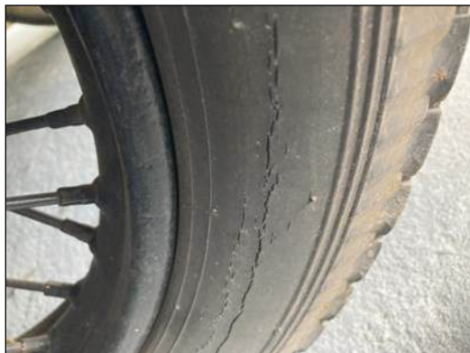
Too cracked for me
