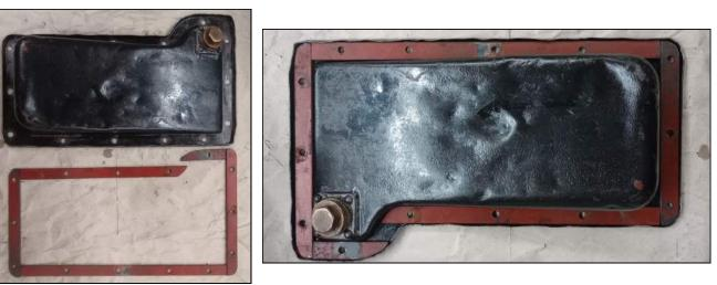
The kit is made up of 5 pieces of flat mild steel approx. 20mm wide and 2-3 mm thick drilled to match the holes in the sump. I bought the kit at an autojumble some time ago, but it would be quite easy to make one using the sump as a template.
