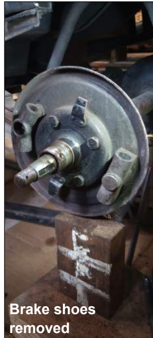
Axle pin withdrawn
