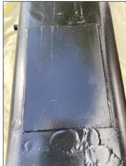
Showing extra plate welded over pinhole in tank.
