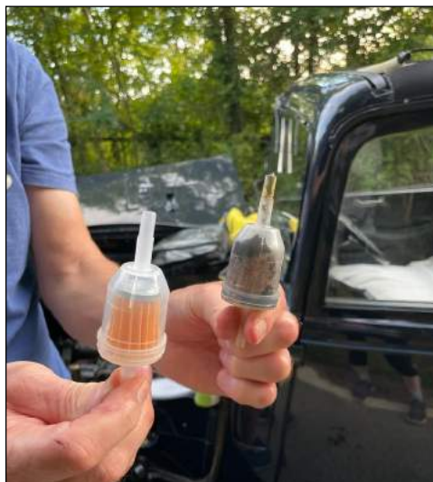
Fuel filters - old and new!
